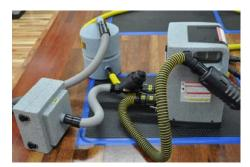
STEP 1: (Left) Install the Interceptor Air In and Out hoses onto the HP unit (as instructed in the Interceptor manual). Remove the Main W from the end of the Air In hose and thread the male end of the Water Separator's hose into the female fitting on the end of the Air In hose.
