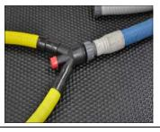
Temporarily attach the Main W with a HB300 (sold separately). Insert the barbed end into the end of 2" truckmount/portable suction line.
