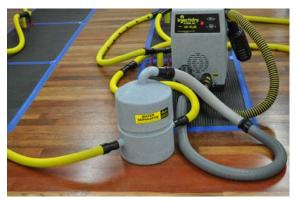
STEP 1: (Left) Remove Main W from the end of your AIR IN main hose (either HP60 or HP-PLUS).
