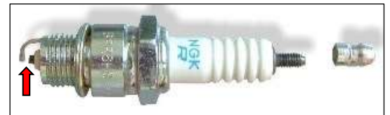
Space between electrodes : 1,5 – 2,0 mm
