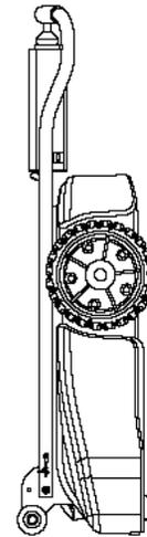
Secure the Rover's urethane plastic traction wheels against wall and then strap into place.
