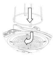
2. Slide HEPA filter element down over filter frame. Ensure filter is centered over the Velo air intake. 3. Pull prefilter cover down over HEPA filter element.
